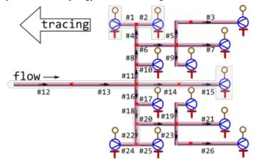
Tracing starts from sensor-equipped nodes and goes backwards, i.e against the flow direction.
